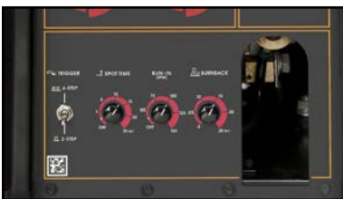
Timer Functions Adds 4-step trigger interlock, spot mode, adjustable run-in speed for smoother arc starting, and adjustable burnback time to minimize wire sticking in puddle.
