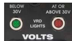
VRD portion of nameplate with green light on.
